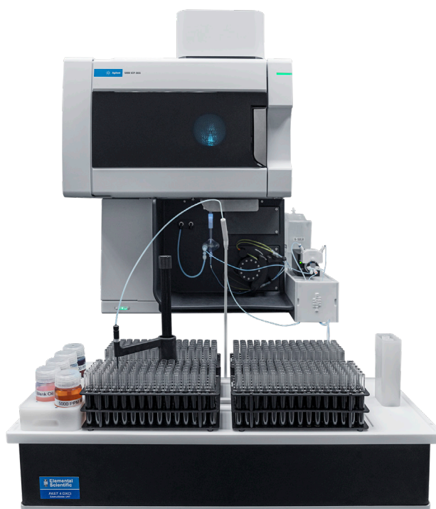
Figure 3. SampleSense FAST UHT-O on the Agilent 5900 ICP-OES with four 90 vial racks and a 4DXCi (2F-SS-Oil-65). Autosampler options also include 2DXCi, 8DXCi, and 14DXCi.
